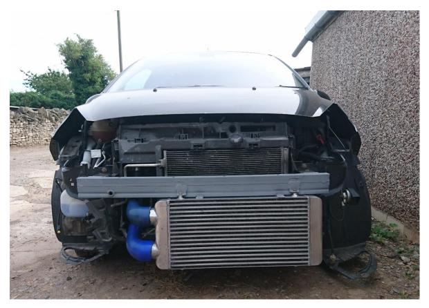
The lower outlet requires a 76 to 51mm 90 bend. A 45-degree stainless 51mm tube can now be used to weld a mounting boss for the MAP sensor and the temperature sensor. The air doser valves can be removed as they are very small and restrictive.
