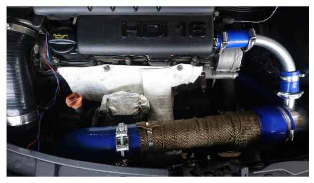
Here's the down pipe after wrapping with titanium heat wrap. A tip here is not to use the cheap metal cable ties, but buy a couple of drive shaft clamps. These hold the heat wrap on well and don't come loose. Another tip is not to rub this heat wrap all over your skin, it's VERY itchy stuff.
