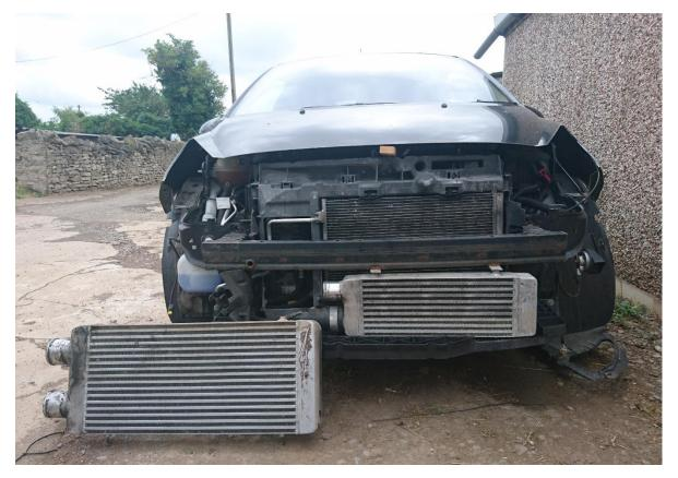
Surprisingly this monster intercooler fits beneath the bumper on the 207 without any cutting required. Mounting brackets can be welded directly on to the steel bumper support beam. Here I sprayed with some primer after welding but painted black afterwards so it would not show through the bumper.
