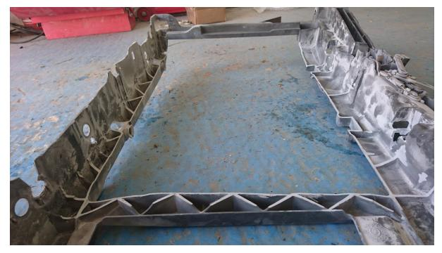
Two holes can be drilled in the base and then the radiator slotted back in, this holds it perfectly tight and gives much more room. The top can be held in using a couple of bolts through the plastic. Ignore the dents on the radiator, this was from the initial attempts to fit the turbo in, clearly it wasn't going to happen.
